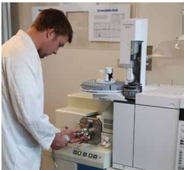
Brad Lewis operates the accurate-mass time-of-flight spectrometer, which can rapidly identify the presence of chemicals of interest. Photo: G. Vaughan, OEH.
