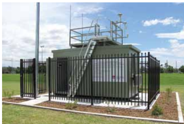
The new air monitoring station at Singleton will provide real-time information on air quality in the region. Photo: OEH.
